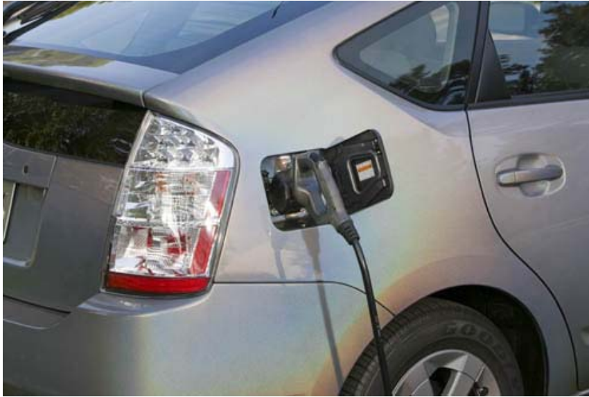
Figure 7. The Toyota Prius is an electric hybrid that provides substantial gains in fuel economy and major reductions in total tailpipe emissions. It uses 0.64 kWh of energy per passenger-mile (given typical vehicle occupancy).
