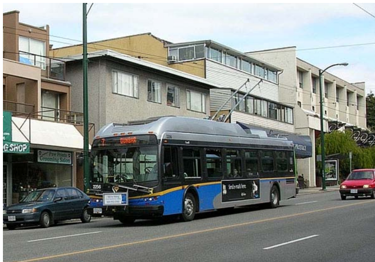
Figure 4. A trolleybus in Vancouver, BC is powered by overhead electrical wires therefore eliminating any tailpipe emissions. A trolleybus uses 0.36 kWh of energy per passenger-mile (given typical occupancy).
