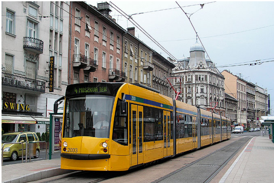
Figure 3. The modern Combino tram uses 0.11 kWh of energy per passenger-mile (given typical vehicle occupancy).
