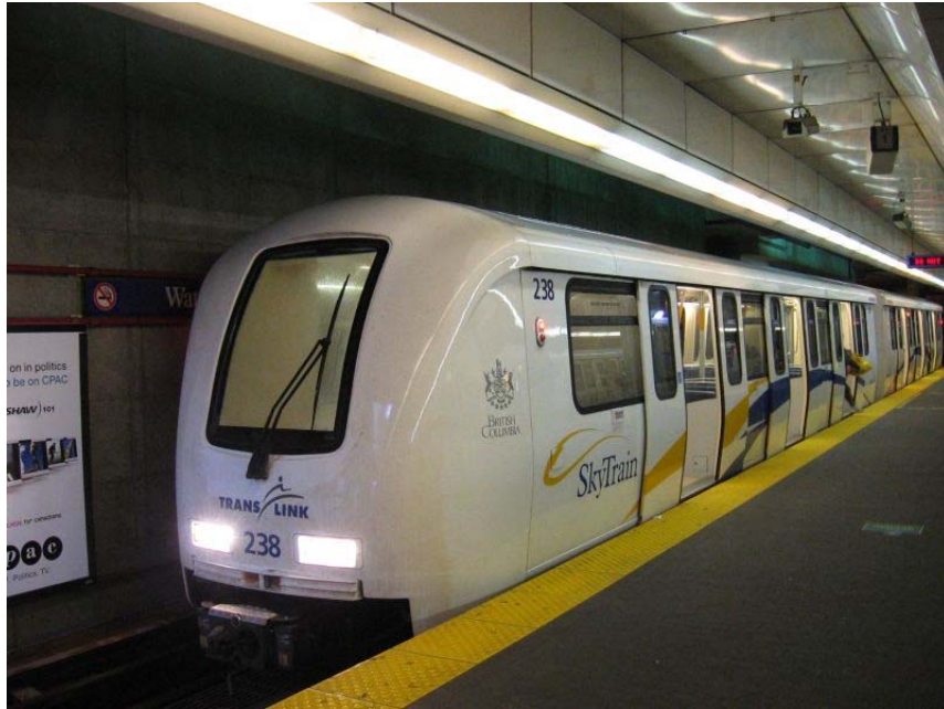
Figure 5. The skytrain in Vancouver, BC uses 0.30 kWh of energy per passenger-mile (given typical occupancy).
