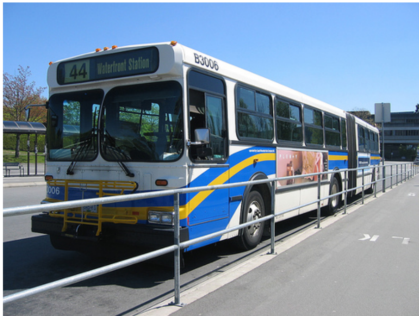
Figure 6. Shows an articulated diesel bus in service in Vancouver, BC that uses 0.56 kWh of energy per passenger-mile (given typical occupancy).
