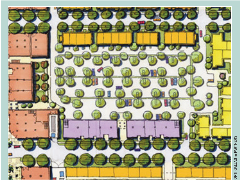
In regards to retail, it's all about the parking. The ideal solution is to bury the parking so the pedestrian realm is not sacrificed. To address this issue in the plan for Baldwin Park in Orlando, Fla. (shown above), a surface parking lot is surrounded by commercial uses on one side of a 300-foot by 600-foot block and residential uses on the other three sides. In blocks of larger sizes and higher density uses, structured parking replaces the surface parking lot.
