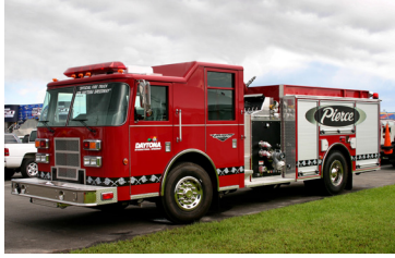
Side-mount pumper, Daytona, FL. Credit: Oshkosh Corporation.
