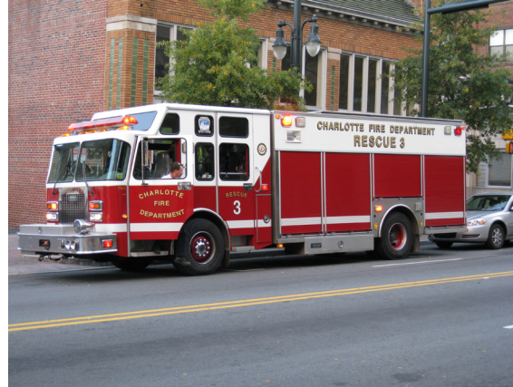
Charlotte, NC Fire Heavy Rescue truck with roll-up cabinet doors. Credit: Patrick Siegman.
