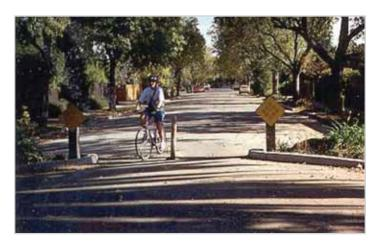
Figure I Traffic calming techniques-street closed to cars only
